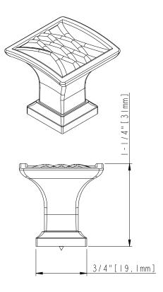
ACCESSORY: SCREW:8-32XI-I/8" IPCS BREAK AWAY SCREW: 8-32x45 IPCS ALL SCREW MATERIAL: STEEL-SAE1006
